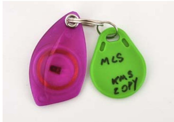
KMS Sharktooth (EM4002) – 125kHz RFID
