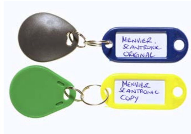
Menvier/Scantronic – 125kHz RFID. Part ref: PROXTAG (PK5)
