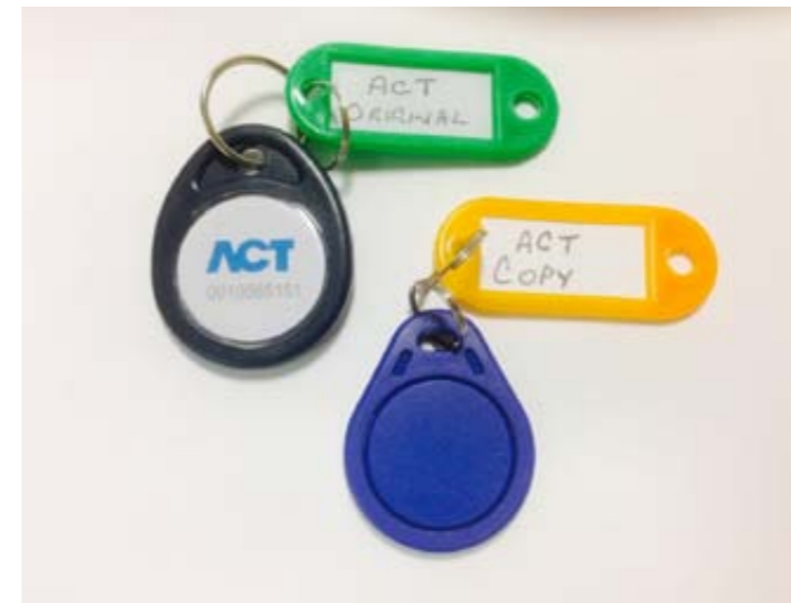
ACT proximity fob, 125KHz RFID (marked with company logo and ID number).
