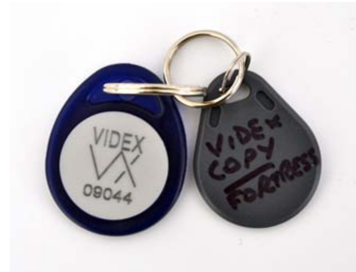
Videx 955/T (EM4002 / 32 Bit) – 125kHz RFID
