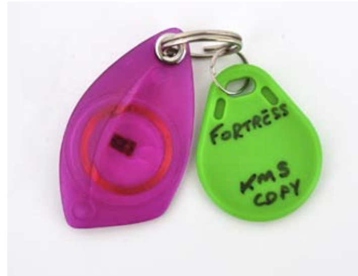
KMS Sharktooth (EM4002) – 125kHz RFID
