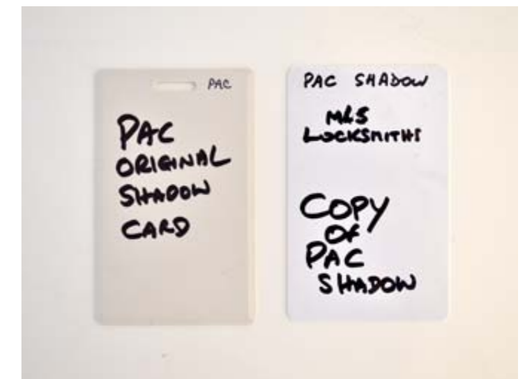
PAC "Shadow" Card ISO — 125kHz RFID
