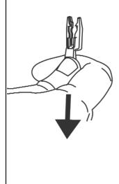
Hold the breakglass as shown and, using medium force, push up with both thumbs simultaneously. You will see the yellow activated band disappear and will hear a click. If the unit now looks like picture no 1, you have correctly reset the breakglass unit. Now check that the door has relocked.
