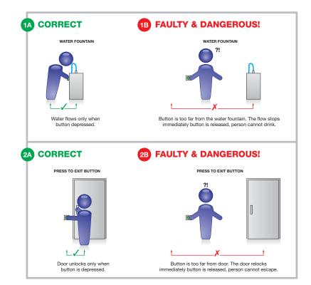
ALWAYS CHECK THAT WHEN A BUTTON IS PUSHED <u>AND HELD DOWN</u> THE DOOR STAYS UNLOCKED AND DOES NOT RE-LOCK. ALL INSTALLATIONS MUST COMPLY WITH BUILDING CONTROL REGULATIONS.
