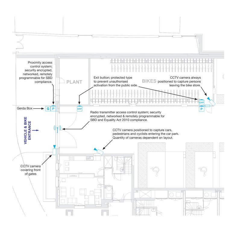
An automated entrance used by both cars and cyclists requires both radio access control for cars and proximity access control for cyclists.
