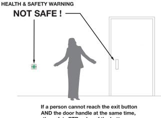
AND the door handle at the same time, the safety PTB poles of the button are USELESS. The installation is unsafe and dangerous.
